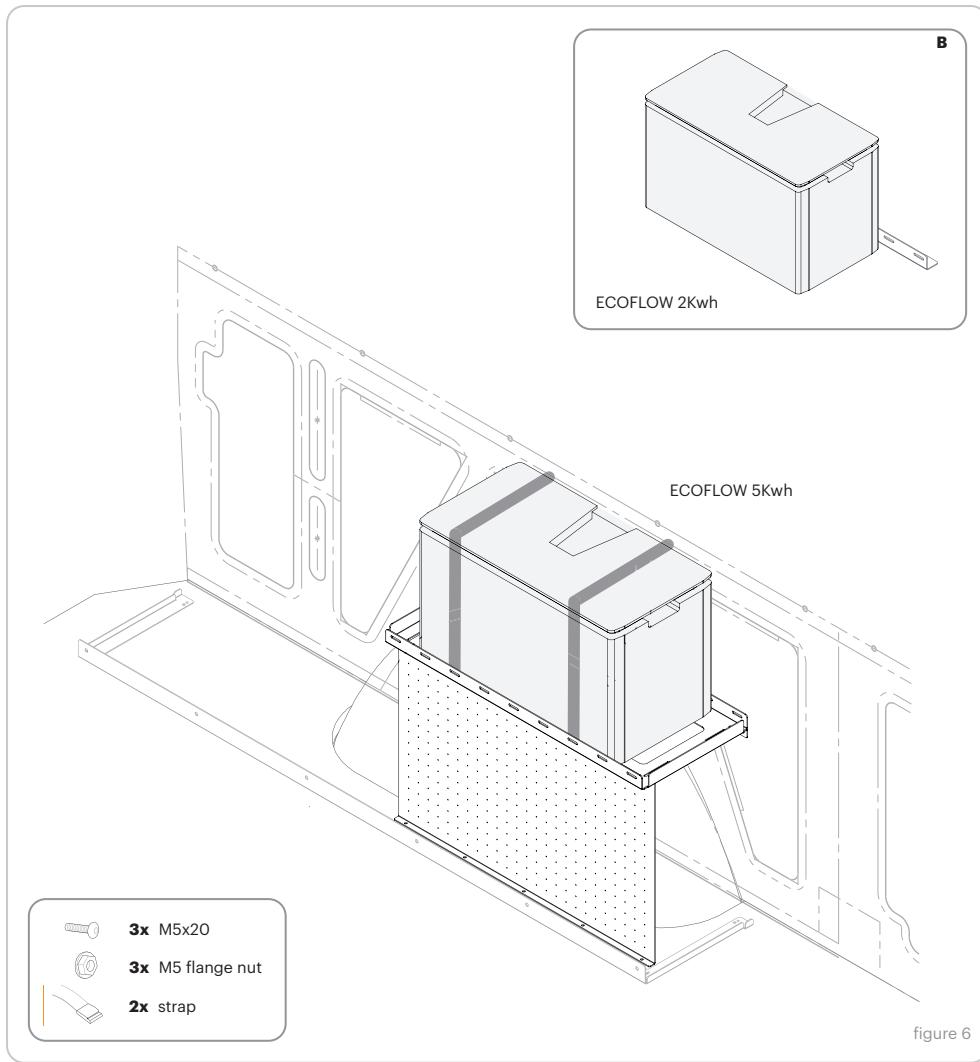
**3.** The battery bracket is able to fit most battery brands, however this example demonstrates the 5kwh and 2kwh batteries from the ECOFLOW independence kit. The slightly smaller 2kwh battery leaves additional room at the backside
