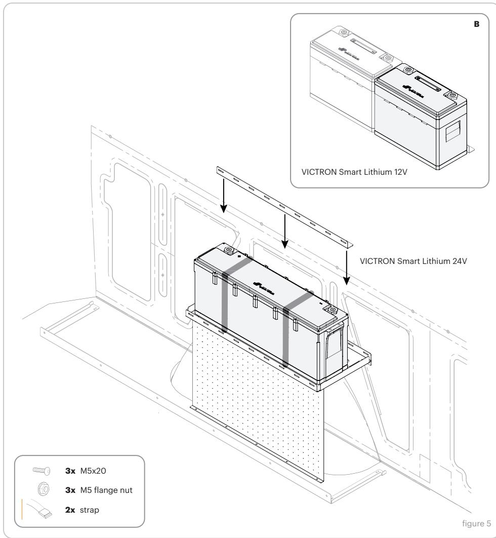
**3.** The battery bracket is able to fit most battery brands, however this example demonstrates the VICTRON smart lithium series. Due to the thinner size the battery can be mounted either at the front or at the back.
