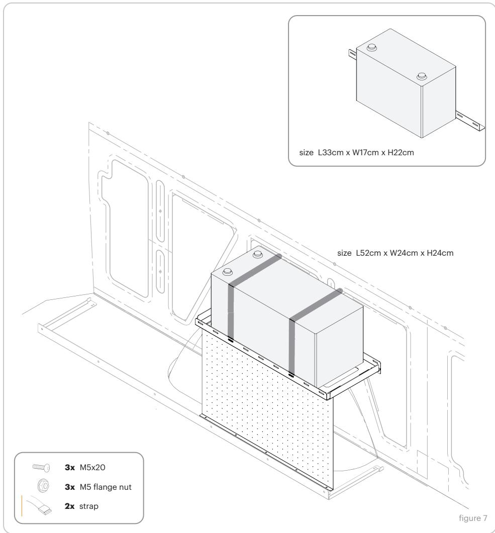
**3.** Here is an example the most commonly found universal battery sizes. When using a smaller battery there is extra room at the backside for additional electrical infrastructure.
